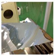
Developed a special machine just for long foils. It continuously supplies foil to the lapping machine to polish. After the polishing, it automatically rolls it up again.
